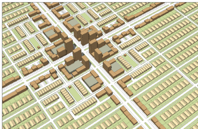
The Miami 21 citywide form-based code guides development for transition areas between high rise structures at transit nodes and relatively low density residential areas. (Source: DPZ)
