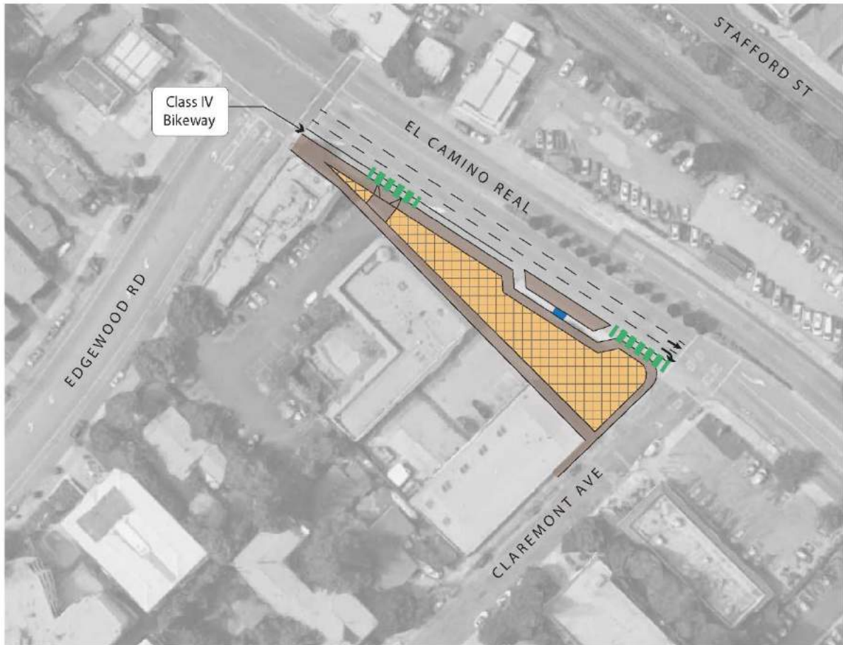
Figure 1: New Configuration for El Camino Real/Edgewood Road/Claremont Road Intersection
